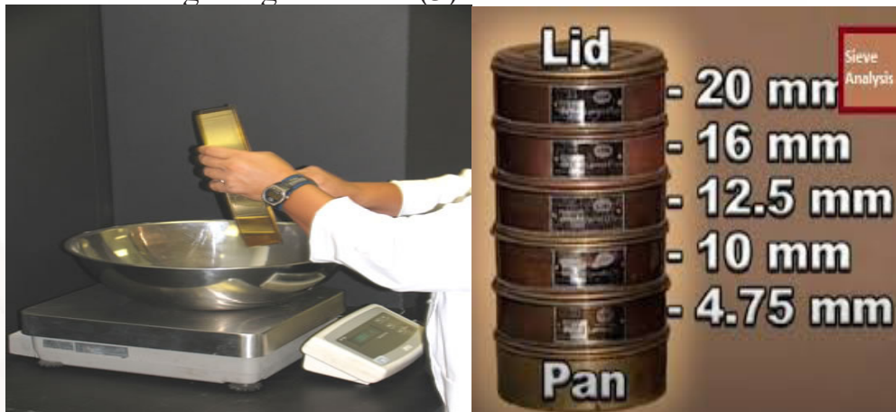
Figure (3). A set of standard sieves are suitable for the classification of loose sediments.
