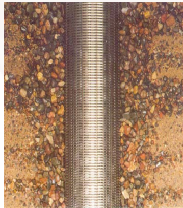
Figure (2) Natural development removes most particles near the well screen that are smaller than the slot openings, (4).
