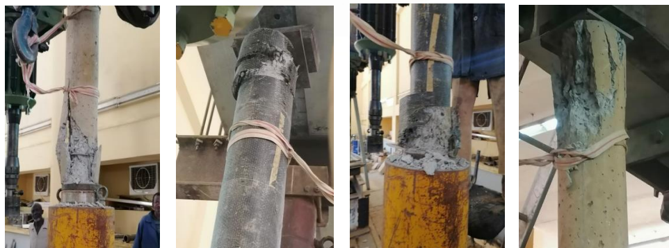
Figure 3. Mode of failures for tested columns.
