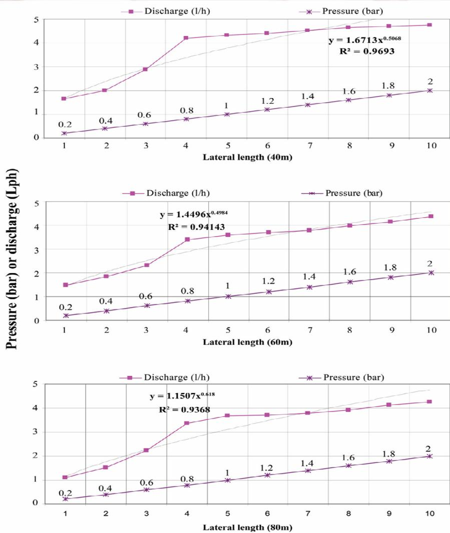
discharges of the closed circuits connections (CM2DIS) type when slope 0%.
