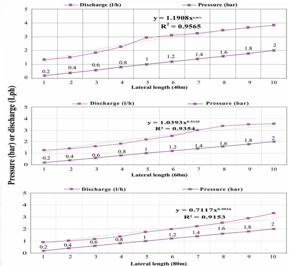
**The Selected Drippers on the lateral lines of (CM2DIS)** discharge can't decrease, Absolutely. When used CM2DIS connection method at all lateral lengths 40, 60, and 80 m the PVEM was 0.6 bar, and under CM1DIS, with all lateral lengths treatments 40, 60, and 80 m the PVEM was 0.8 bar, while the traditional drip method at all lateral lengths 40, 60, and 80 m the PVEM was 1.0 bar.
