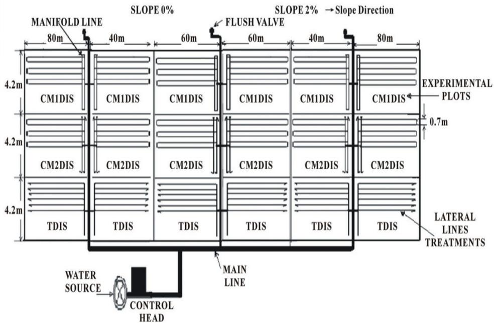
**Figure 7.** Layout of the experimental plots: Treatment L = 40 m; L = 60 m and L = 80 m different Field conditions Slope 0%; Slope 2% levels.
