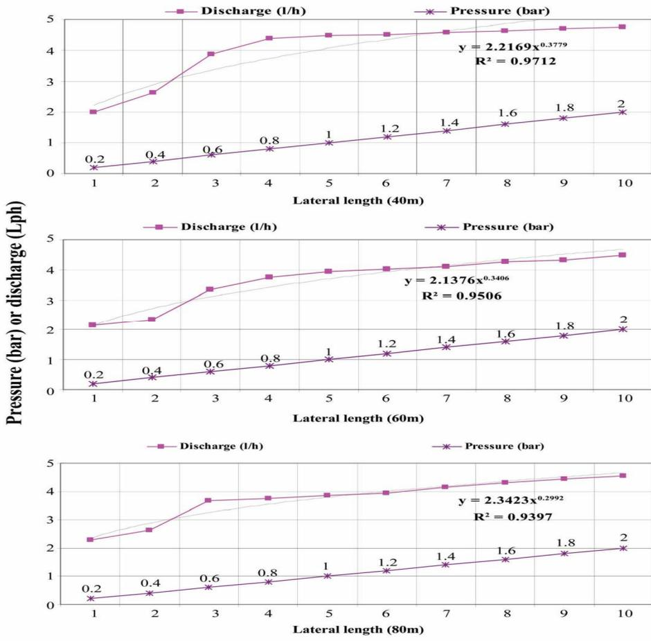
discharges of the traditional drip system (TDIS) when slope 0%.
